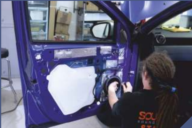
Tom fitting the front door Audison VOCE II AV K6 S woofers with Skinz sound deadening & Water Guard
