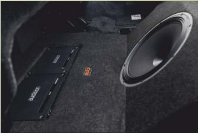
The boot, with Audison amps and 12" subwoofer
