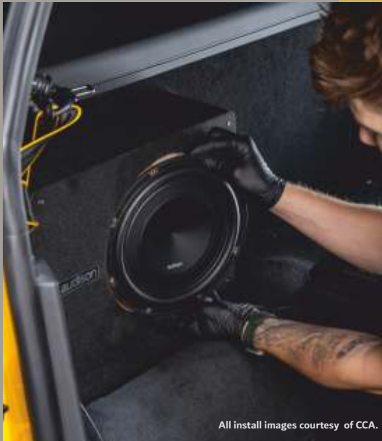
AUDISON Prima active sub installation.
