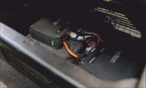
Audison DRC mounted in the centre console to control the FORZA amps
