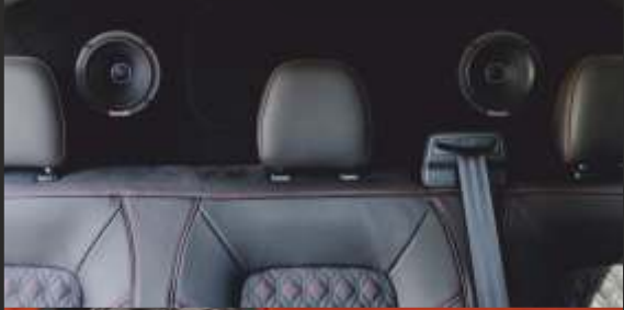
Audison Voce II AVX 6.5 Coaxials mounted in the rear seat bulkhead
