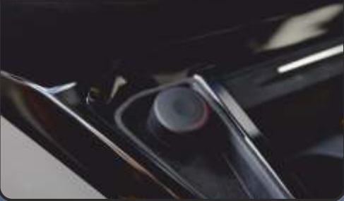
Audison DRC mounted in the centre console to control the FORZA amps
