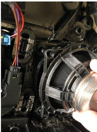
Place the new Eton midrange driver with the 3 fixing lugs centred on the rubber holders and press all 3 in succession until you notice that the loudspeaker is engaged.
