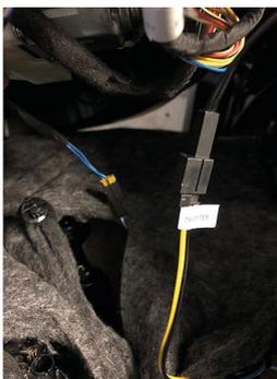
the midrange driver into the connector of the mid-range driver.
