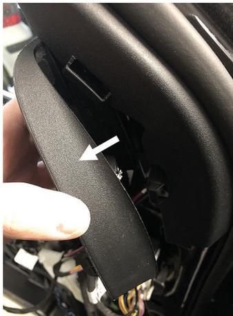
Now disassemble the plastic mirror cover which contains the tweeter mount.
