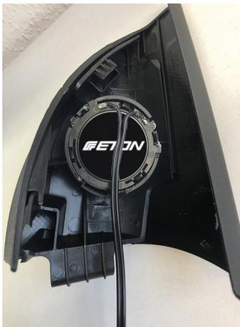
installed at the factory so that the Eton tweeter can be clipped in directly. If you install an Eton MB 100 RX system, there is no need to disassemble the tweeter.
