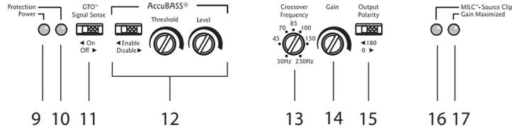
**9. Power LED** – If you have connected your battery power, vehicle ground, and turn-on lead (or GTO signal sensing) correctly, then this light should be green to indicate the power is ON. An internal blue glow will also emanate from the heatsink area to indicate that the power is ON. There are times when this blue glow will flash, such as during power-up, and when the protection circuits have detected a problem.
